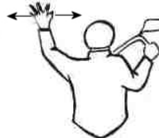
Open Up The Gap Keep stagger as is Wave fully open hand
